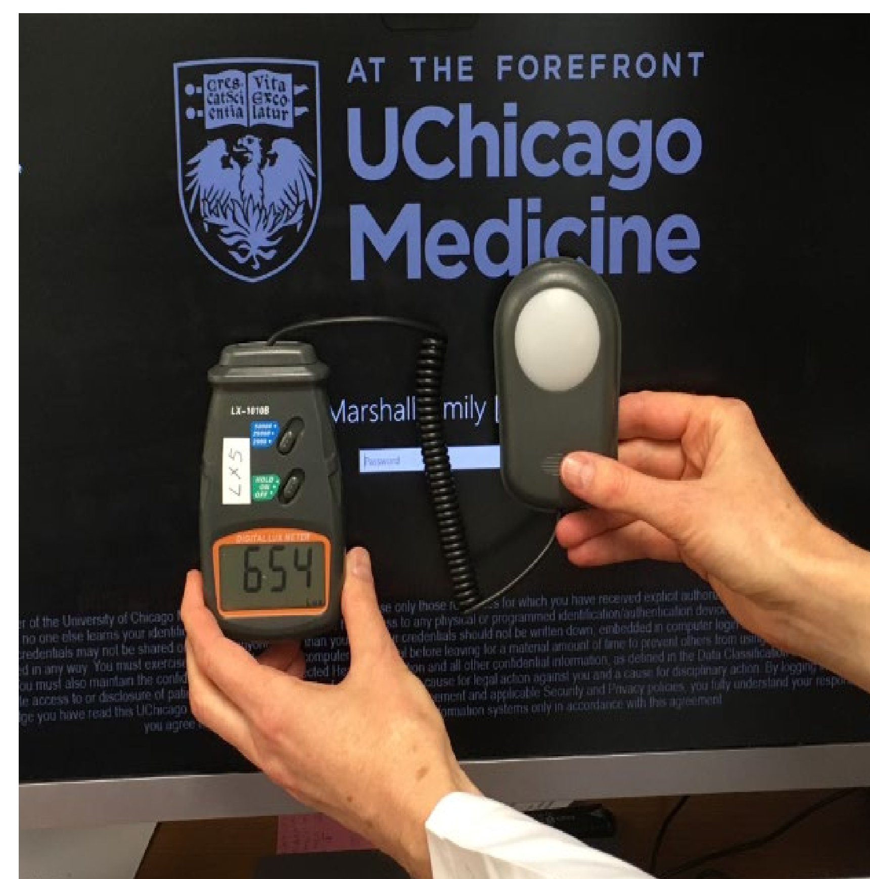
Figure 2. Example of measuring ambient light with an inexpensive photometer calibrated with an in-house photometer with NIST-traceable calibration.
