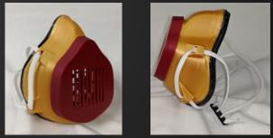
D-profile weather stripping was adhered to the mask lip using a hot glue gun. This prototype technique was further adapted in later iterations to allow for altered fits for different face shapes.
