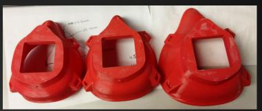
Masks underwent CAD design modifications to produce small, medium, and large versions. Different sizes maintained the same nose cap and hatch pieces, thus allowing for interchangeability of parts
